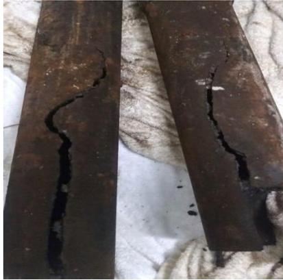
The cast iron pipes have started to fail by cracking and leaking causing a plethora of issues. This is an on-going issue. We will tackle them as needed.
